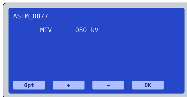
Figure 4 Setting the maximum test voltage, ASTM D877 shown
