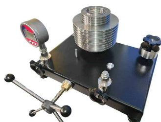
Weight stack loaded and a gauge under test. Reference lines on the column set the working position on DWT-6 to DWT-1600; the DWT-2500 has a digital piston position indicator instead.
