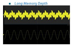
With a maximum memory depth of up to 100 Mpts, GPS-2000HD series is suitable for observing and analysing long-duration signals, low-frequency signals, and transient phenomena. With large memory depth, the oscilloscope is able to process more data, and the accuracy and stability of the calculation results are also much higher.
