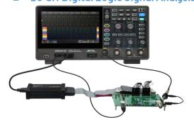
The GPS-2000HD can be used with our 16-channel logic analyser probe option (SLA1016) to add 16 digital channels to the instrument without affecting other test functions, realizing mixed-signal acquisition and analysis, and quickly solving analog-digital mixed-signal design and analysis problems.
