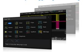
The GPS-2000HD series has a variety of triggering types, including edge, slope, delay, set/hold, and a variety of bus triggers (serial triggers). It supports triggering and decoding of I2C, SPI, UART protocols in the embedded industry and CAN, LIN protocols in the automotive industry, and can accurately capture and intuitively display the protocol information of the bus in a table or in other ways, so that it can be tested with stability.
