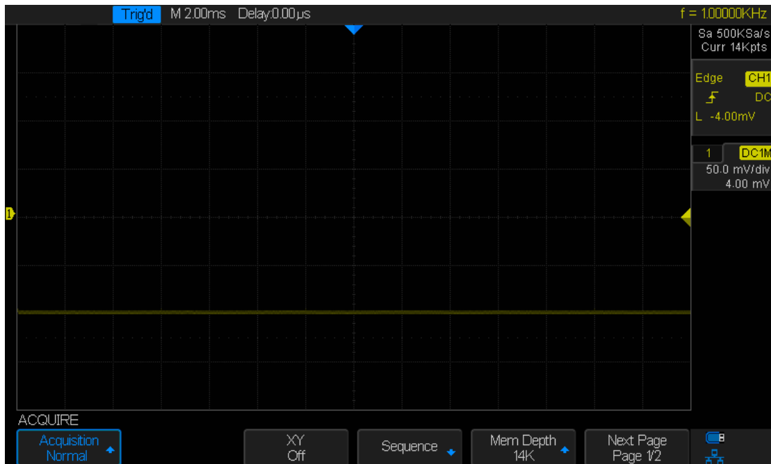
Figure 15 Pulse With 0.1% Duty, Normal Mode
